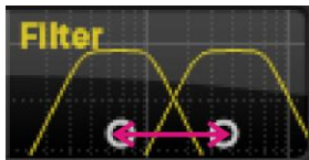
Moving the white dot horizontally changes the filter frequencies in the same direction, moving the frequency pass-band higher and lower
